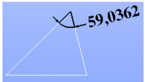
**Angle** can be shown for two intersecting edges or three points
