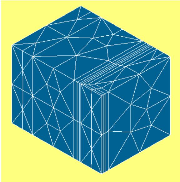
It has become possible to specify wall faces, which are not the inlets and outlets, and faces shared by solids as target faces for **Viscous Layers** hypothesis and create viscous layers on them.
