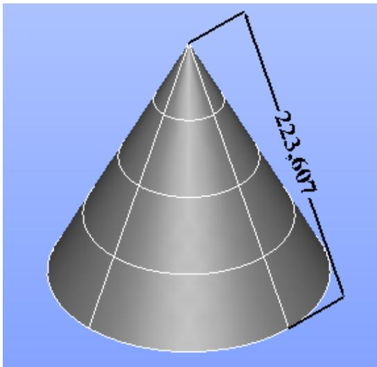
It is possible to display the **Length** of a single edge or **Distance** between two vertices or two parallel edges;
