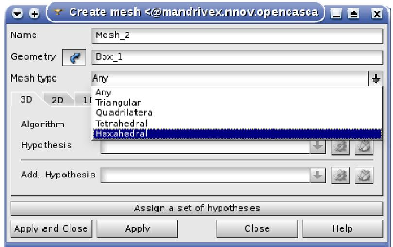
**Default** is shown instead of **None** if an algorithm can work without any hypothesis using default parameters.
