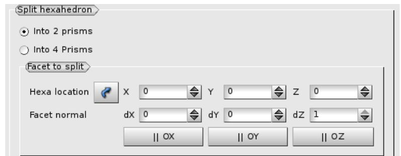
Then it is possible to choose the side of hexahedron that will be split into triangles by specifying a point and a direction close to normal of the side.
