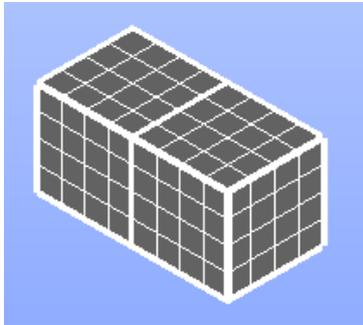
New **Remove Extra Edges** option of **Fuse objects** operation allows automatically removing edges of argument objects from the operation result.
